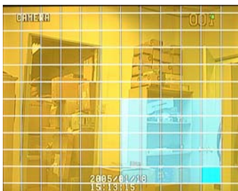
When Select Multi Region, Using Direction Key in ② to Expand Non-Activate Region
